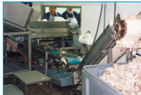
Workers on the pet food packaging line stand on a raised GatorGrate work platform (on adjustable pedestals) using an entire 4-foot by 12-foot panel. The raised platform expedites the frequent washdowns that are required. Any debris that falls on the grating is easily hosed off.
